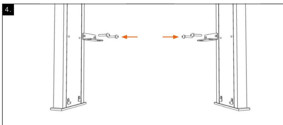
All fixing brackets are lacquered according to the colour of the shelf/box. Screw the appropriate fixing brackets at the required positions onto both sidebars and tighten them firmly.
