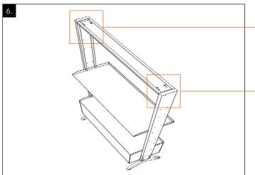
**Mounting crossbar:** Screw crossbar onto the sidebars and <u>fix it firmly</u> on each side.
