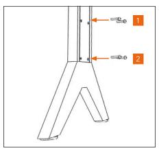
Tighten all 4 screws firmly (1) and (2), if there is <u>no shelf/box</u> planned for the 2 lowest levels.
