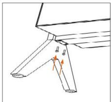
Screw it with <u>loose fitting</u> from the bottom.
