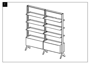
**Final fixing:** Finally tighten all screws with loose fitting underneath the shelves/boxes.
