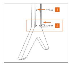
Attention: If a shelf or a box is planned at the 2 lowest levels, screw the apropriate fixing bracket now firmly onto the sidebar (2).
